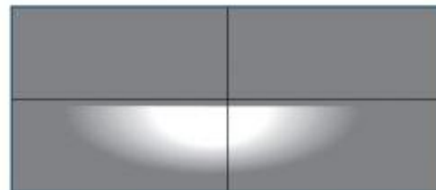
Modern symmetric dipped beam headlamp pattern on light board
