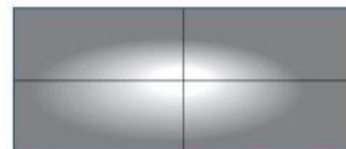
Main (high) beam headlamp pattern on light board
