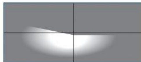
Asymmetric dipped beam headlamp pattern on light board
