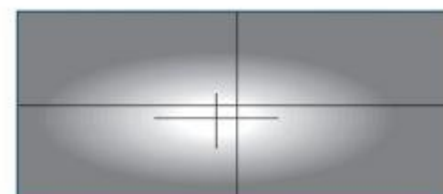
Older-style symmetric dipped beam headlamp pattern on light board
